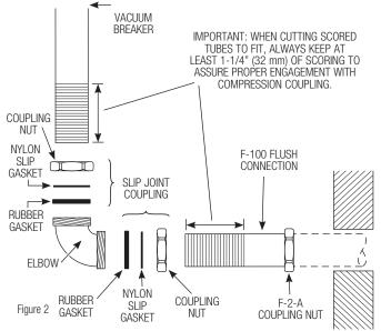
**IMPORTANT:** Before inserting the scored ends into the Elbow, apply several drops of Loctite (supplied by Sloan) to the scored ends of the tubes (Figure 3). This sealant helps prevent separation under high-pressure conditions. **DO NOT** use any other pipe sealant or lubricant on this connection.
