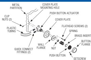
Using Cover Plate as a template, drill two 3/16" (5 mm) Cover Plate Mounting holes and cut opening for Push Button Actuator into the metal partition. Install Clip Nuts with threaded side toward back. B) Insert threaded end of Push Button Actuator through Cover Plate and Wall Flange and install Nut. Tighten Nut securely.
