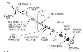
A If not already completed, bore a 1-1/2" (38 mm) diameter hole in wall for the Push Button Actuator. Refer to the Rough-in drawings on Pages 2 and 3.
