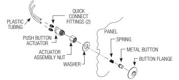
Attach Plastic Tubing to Push Button Actuator. See: Steps to Attach Plastic Tubing (below).
