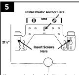
Measure and mark rough in. If in-wall carrier is not used. Use a 5/16" masonry bit to drill hole, then install the hanger bracket with one plastic anchor and screw.
