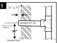
Set drain line height 16" from finished floor (standard 24" rim) or 9" Max. for ADA installation. Threaded nipple should extend 1/2 to 3/4" from wall. \*IMPORTANT Nipple must not extend more than 3/4" past the finished wall
