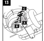
**Connect battery A to wire B.**Wait 1 minute for system to start up. Note system will allow 2 manual flushing before pausing 30 seconds.
