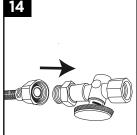
Put adaptor onto stop then attach supply line to adapter. Turn water on and assure there are no connection leaks.
