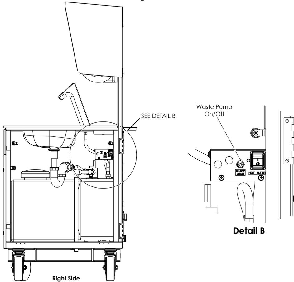
1. Drain the waste tank (Electric Pump).
