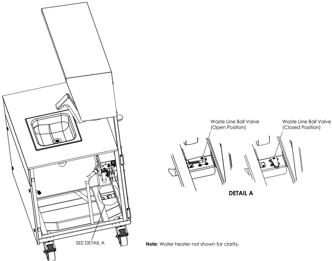
1. Drain the waste tank (Gravity Fed).
