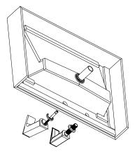
5. Install Faucet and Soap spouts, (Figure 5) onto sink according to manufacturer's instructions provided with component.
