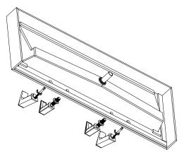
5. Install Faucet and Soap spouts, (Figure 12) onto sink according to manufacturer's instructions provided with component.
