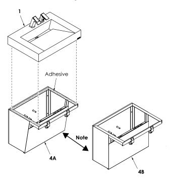
**Note:** Angled Enclosure and Vertical Enclosure, sink installation is the same.
