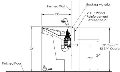
Note: Backing material should equal thickness of drywall, 1/2" min.
