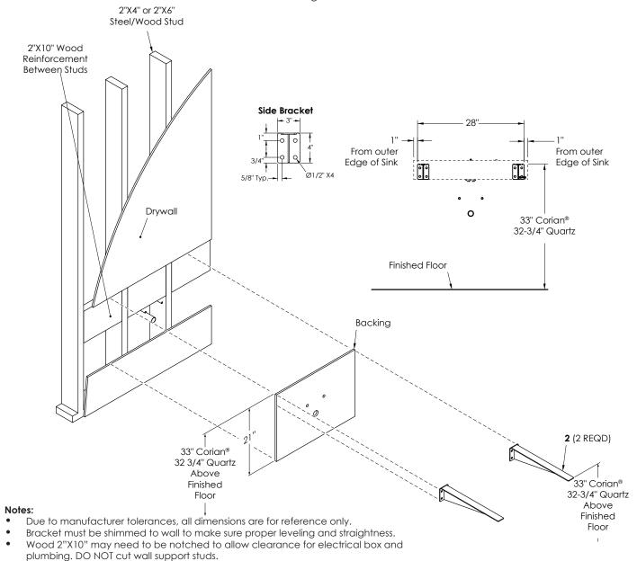
1. Install Backing Figure 3 onto wall studs.
