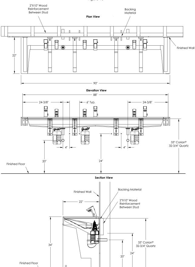
Note: Backing material should equal thickness of drywall, 1/2" min.
