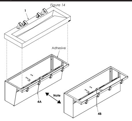
**Note:** Angled Enclosure and Vertical Enclosure, sink installation is the same.
