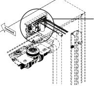
PCB CONTROL BOARD Located on the back of the Bottle Filler Housing
