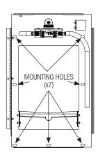
Secure unit to wall with appropriate mounting hardware (not provided).
